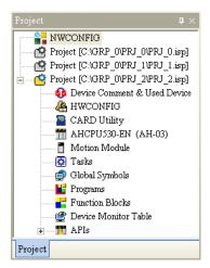
(3) If there are projects for AH500 series CPU modules, the users have to open the HWCONFIG windows in the projects, and complete hardware configurations. The users have to configure modules, set the parameters in network modules, gives names to the CPU modules, set ports, and set Ethernet ports. Please refer to chapter 3 for more information.
