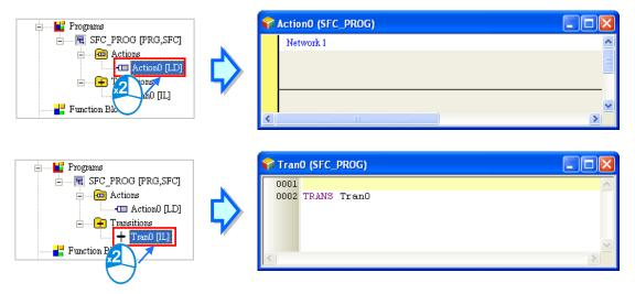
\*. If the transition create is assigned to a transition in the sequential function chart, the window for the transition will be opened after users double-click the transition in the sequential function chart.
