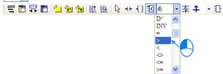
(2) Select a line, a contact, or a group of devices. Before users connect a comparison contact to a group of devices in parallel or in series, they have to draw a frame round the group of devices. After users make sure of the position in which a comparison contact will be inserted, they can click on the toolbar.
