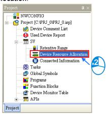
Users can set a device range in the **Device Resource Allocation** window. Every type of device has its limitations. For example, the data registers in a DVP-SV series PLC start from D2000, the auxiliary relays start from M2000, the counters are 16-bit counters, and the timers take 100 milliseconds as the timing unit. If users select a device address which is not allowed, the system will modify it automatically.
