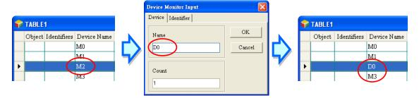
Users can click the Identifier tab and add identifiers in this Device Monitor Input window.
