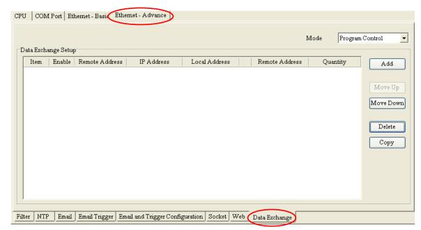
If users open this page of the PLC Parameter Setting window for the first time, the table is blank due to no data set. A new row of data can be inserted by clicking **Add**. Double-click the data so that the data setting window is opened.
