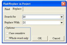
After the users use the **Find/Replace** function, the search results will be displayed in the message display area at the bottom of the ISPSoft window. If the users double-click a search result, the system will lead the users to the position of the object corresponding to the search result.
