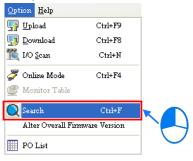
(2) Click in the **Find what** box, select a module in the **Module Selection** window, and double-click the module. The users can also type part of a module model in the **Find what** box. Finally, click **Find**.
