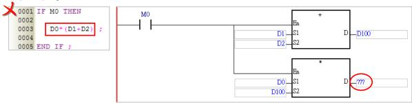
A structured text is composed of statements, and a statement is composed of elements. An example of a structured text is shown below. The complete statements in the structured text are in the red frames.
