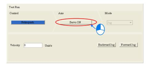
When **Servo ON** is clicked, various test-run modes in the **Mode** field are for option. There are different execution functions for users to type under various modes. The corresponding functions are explained as below.
