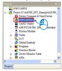
After HWCONFIG is started, the users can double-click the CPU module to open the **PLC Parameter Setting** window. Click the **CPU** tab at the top of the window, and the **System** tab at the bottom of the window.
