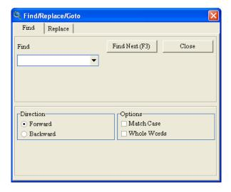
The users can do a search on the object typed in the **Find** box by clicking **Find Next (F3)** or pressing F3 on the keyboard. The users can still do a search on the object typed in the **Find** box by means of pressing F3 on the keyboard even if the **Find/Replace/Goto** window is closed.
