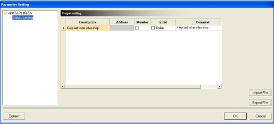
The hardware configuration is not complete until the parameters in the CPU module and AH16AP11R-5A are set. However, the configuration and the setting must be downloaded to the CPU module so that they can take effect. The configuration and the setting are saved here, and will be downloaded with the program in the project later.
