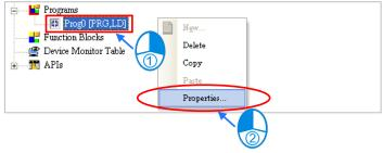
(2) Type the same passwords in the Enter Password box and the Confirmation box, and then click OK. English letters, numerical digits, and special marks can be typed in the boxes. Once the POU is protected with the password, the system asks the users to type the password whenever the window for the POU is opened.
