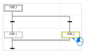
(2) After users click on the toolbar, a jump point will be inserted. The users can also insert a jump point by right-clicking the step or the transition selected and click **Jump to a Step**.
