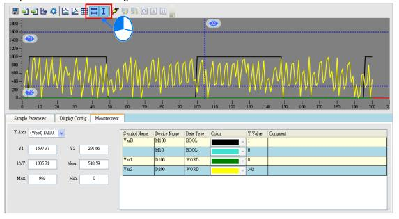
Drag two horizontal measuring lines Y1 and Y2 to the position where the measurement is performed. The values of the horizontal measuring line will display at the bottom of the following figure. After the coordinate of Y axis is selected in the box, the value of the horizontal measuring line Y1 will display in Y1 box and the value of the horizontal measuring line Y2 will display in Y2 box. The value in  $\mathbf{I}\Delta\mathbf{Y}$  box is the difference value between Y1 and Y2.
