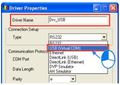
(5) Select a device name which corresponds to the PLC connected in the COM Port drop-down list box in the Communication Port section, select the number of times the sending of a command is retried if a connection error occurs in the Time of Auto-retry box, and select an interval of retrying the sending of a command in the Time Interval of Auto-retry box. Click OK.
