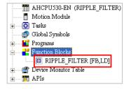
If a POU of the program type wants to call this function block, the users must declare a symbol whose data type is a function block in advance. In other words, the users have to produce an object which takes part in an operation according to the function block definition. The object produced is a function block instance.
